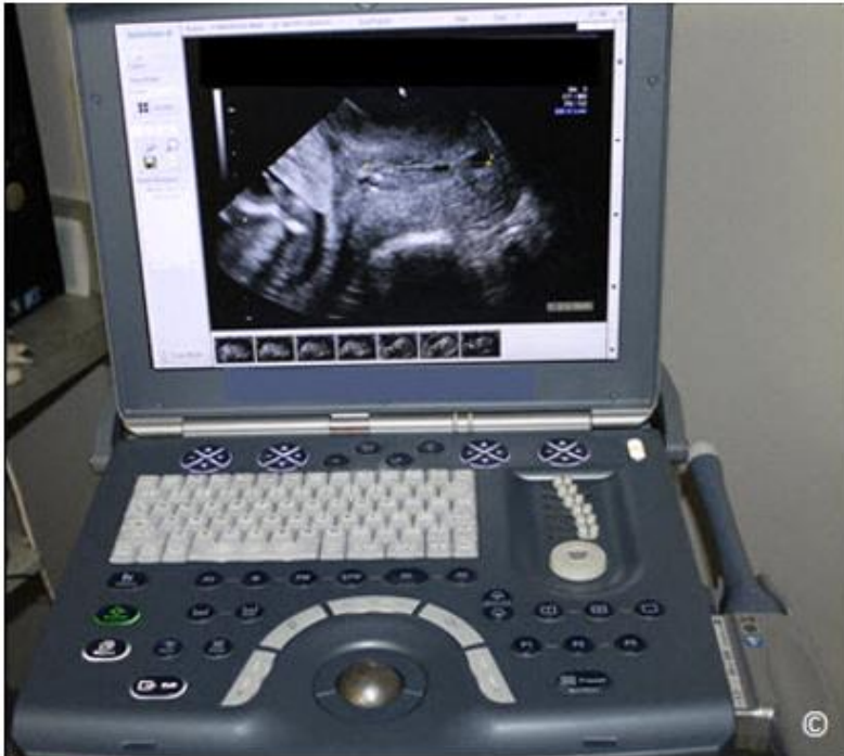
Figure 2.9: Ultrasound equipment showing a wide array of knobs for control of various features. Most ultrasound equipment have a keyboard and a trackball on their consoles.
